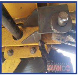
\*Note: On Case Flagship combines, front axle mount and feeder house mount are welded directly in the center of the two existing brackets.
