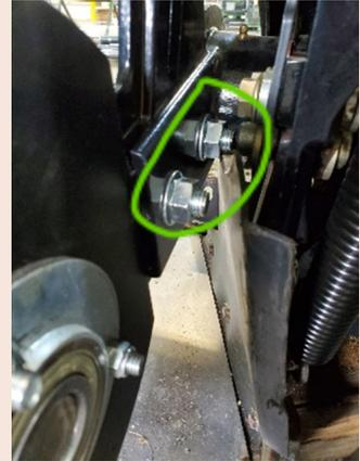
**Step 5:** Using a lifting device again, place the auger into the adapter opening and lift into place. Slide the mounting bars on the idle side and drive side into the mounting brackets, and install four carriage style bolts to hold drum into place.
