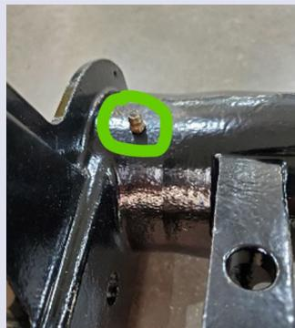
**Step 15:** Remove grease zerck from previously removed drive side mount and install in new drive side mount.
