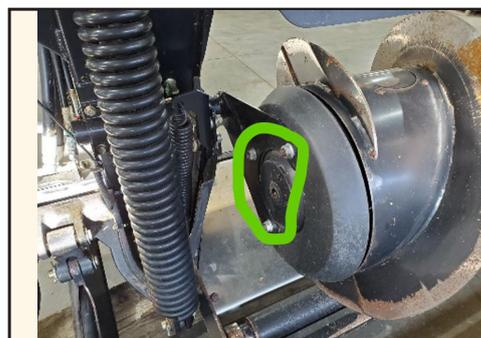
**Step 3:** Remove the 3 nuts from the idle side shown in the picture here.
