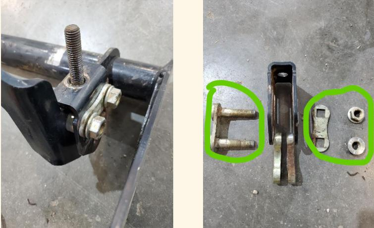
**Step 9:** Remove height adjustment hardware from idle side bracket.
