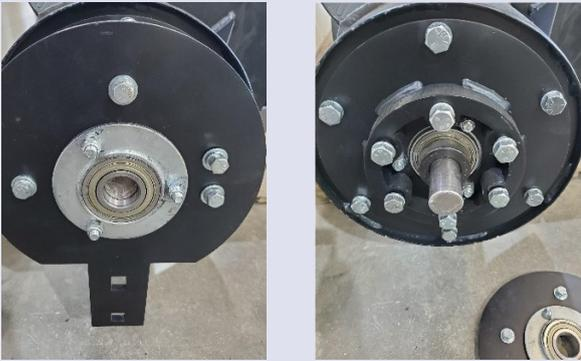
**Step 1:** Remove mounting arm from drive side of drum.
