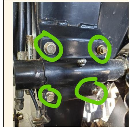
**Step 5:** Remove the 4 bolts holding the idle side mount.
