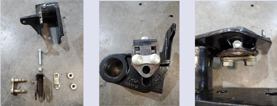
**Step 10:** Install this hardware into the new idle side bracket part# 133503 from the CA20 attachment kit. There is also a 1/2" full thread bolt and lock nut that gets installed into this assembly as well. See picture above.
