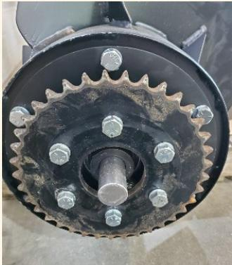
**Step 2:** Install factory drive sprocket to end of drum using supplied bolts.
