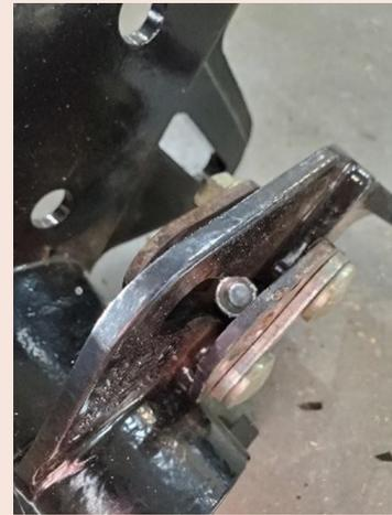
**Step 14:** Install height adjustment parts into new drive side mount part# 279691.
