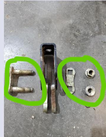
**Step 13:** Remove auger height adjustment parts from drive side mounting bracket. Re-use the same parts as used on the idle side.
