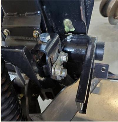
**Step 12:** Install new idle mounting bracket on tube installed in step 8.
