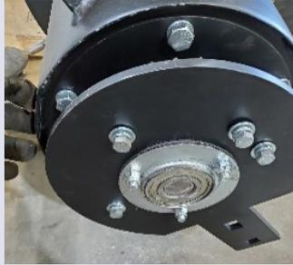
**Step 3:** Slide bearing locking collar on to shaft, then reinstall drive side mount bar previously removed in step #1.
