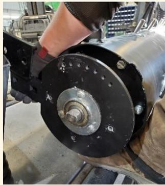
**Step 4:** Remove the idle side cover and timing adjustment lever prior to installing into adapter frame.
