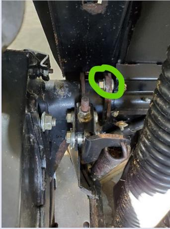
**Step 4:** Remove the 2 bolts and retaining collar from the drive side as shown.
