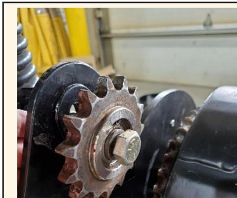
**Step 17:** Remove chain tensioner sprocket from factory drive assembly and install in new drive side mount.
