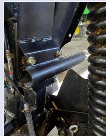
**Step 8:** Install tube on the idle side where bracket was previously removed, using the factory hardware. This tube is included in the CA20 completion kit.
