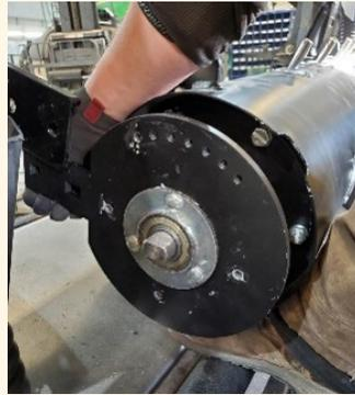
**Step 5:** Remove the idle side cover and timing adjustment lever prior to installing into adapter frame.
