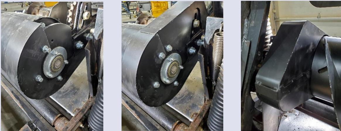
**Step 10:** Tension drive chain, then install chain guards on drive side.
