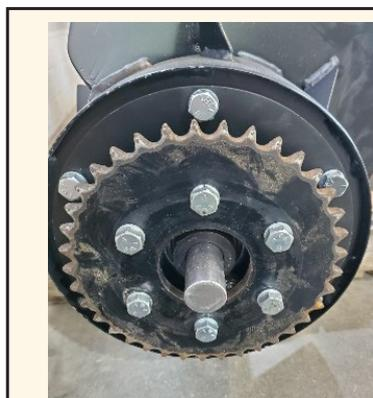
**Step 3:** Install factory drive sprocket to end of drum using supplied bolts.
