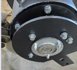
**Step 4:** Slide bearing locking collar on to shaft, then reinstall drive side mount bar previously removed in step #1.
