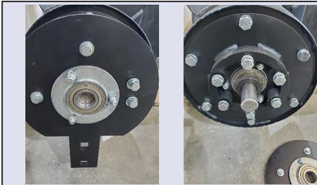
**Step 2:** Remove mounting arm from drive side of drum.
