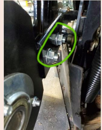
**Step 6:** Using a lifting device again, place the auger into the adapter opening and lift into place. Slide the mounting bars on the idle side and drive side into the mounting brackets, and install four carriage style bolts to hold drum into place.
