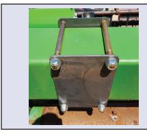
**Step 1:** Install idle bracket assemblies onto back tube of header using four 9" long bolts and nylock nuts. Install everything loose enough so the parts can still be moved by hand when auger is set into place.
