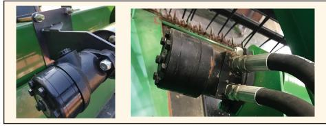
**Step 2:** Install motor assemblies into outside end of each auger. Augers are mirror image; ensure product will be carried towards center of header when auger is rotating in a forward motion.
